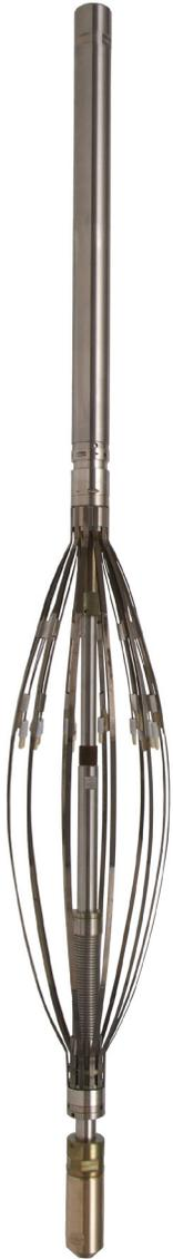
Oil, gas, and water have different dielectric constants. The CAT uses this property to identify fluid phases in high deviation and horizontal wells. Run centralised in the wellbore, the CAT is fully combinable with other Ultrawire\* production logging tools.
