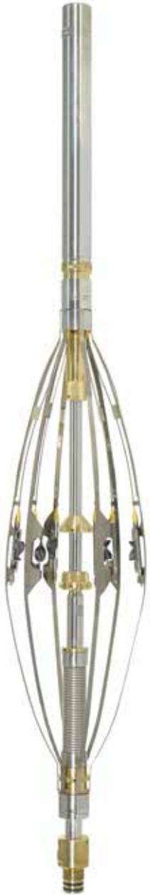
The Spinner Array Tool features six miniature turbines deployed on bowspring arms, enabling discrete local fluid velocities to be measured at 60 degree intervals around the wellbore.
