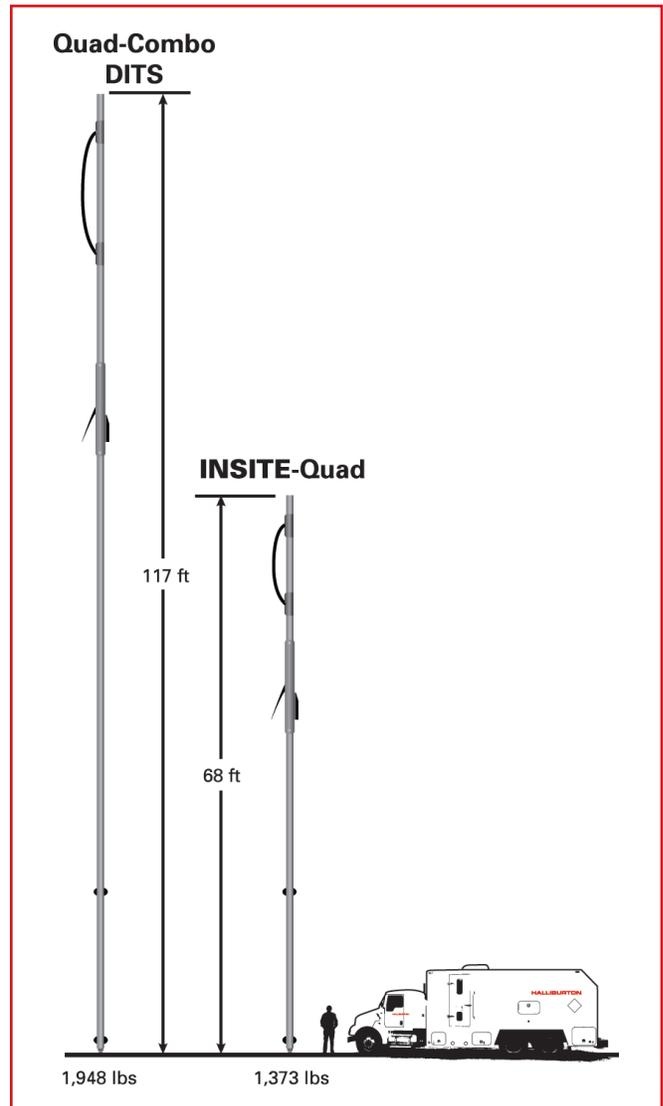
LOGIQ™ INSITE – Quad has a shorter tool string length and faster data transmission compared to the Quad – Combo DITS™.
